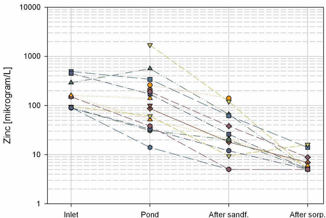
Figure 1. Removal of zinc in the facility in Odense
