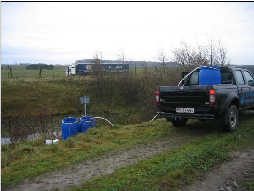
Figure 10 Stormwater is collected from a stormwater pond treating highway runoff.
