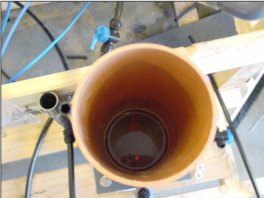
Figure 5: The horizontal and permanently submerged filter applied on laboratory reactor 2 and 3
