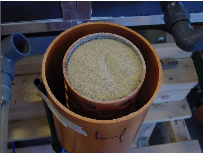
Figure 7: The vertical filter applied on laboratory reactor 4
